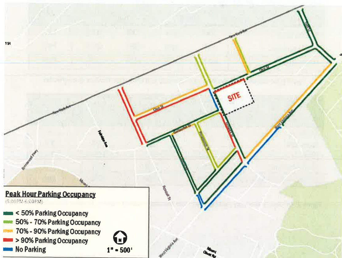
Figure 4: Weekday Peak (PM) Parking Occupancy (Source: Grove/Slade)
