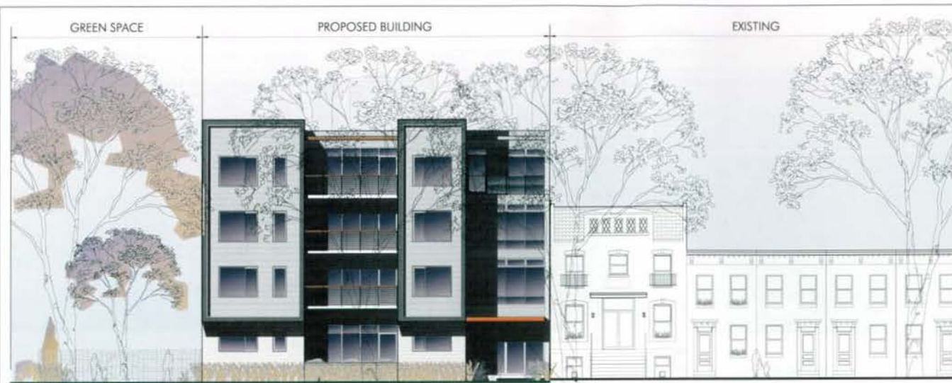
1 SOUTH ELEVATION - FACING RHODE ISLAND AVENUE A2.1 1/8" = 1'-0"
