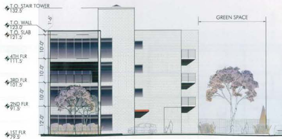
2 NORTH ELEVATION - FACING ALLEY A2.2 1/8" = 1'-0"
