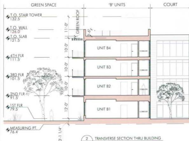
2 TRANSVERSE SECTION THRU BUILDING A2.1 1/8" = 1'-0"
