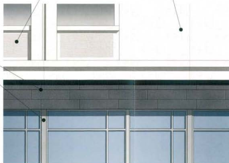
ARCHITECTURAL PRECAST TYPE I ACID ETCHED FINISH
