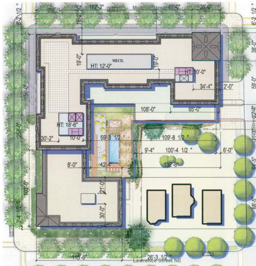
Roof/Building Dimension Plan
