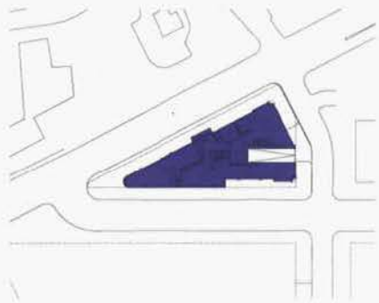
GFA GROUND FLOOR 19,800 SF + 370 SF CANOPIES = 20,170 SF
