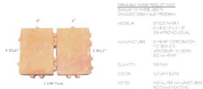
PERMEABLE PAVEMENT PRODUCT INFORMATION Scale: 1/4" = 1'-0"
