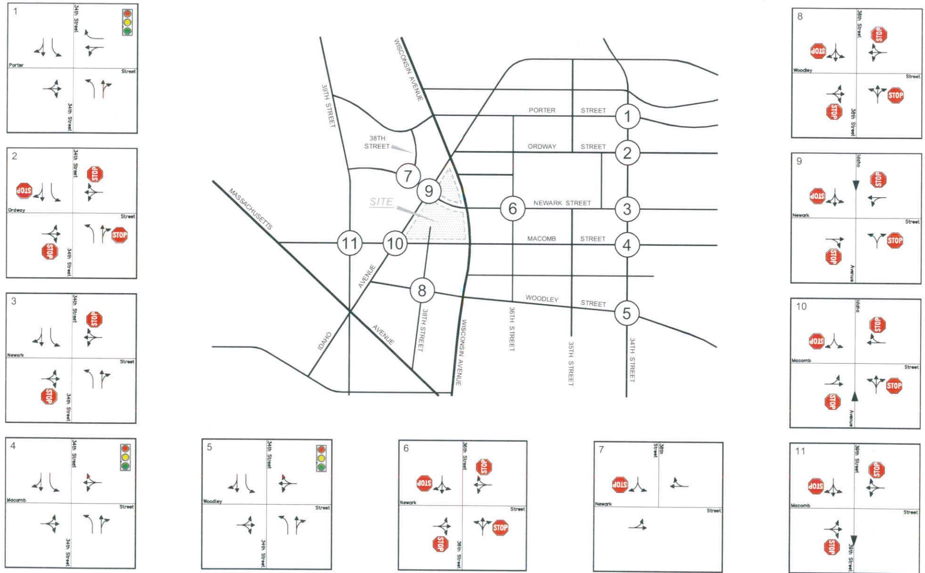
Figure 5-3 Intersection Lane Use and Traffic Control
