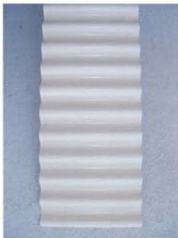
CORRUGATED METAL SIDING
