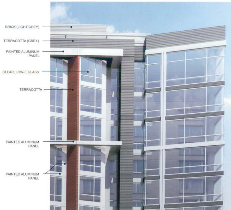
M STREET FACADE DETAIL
