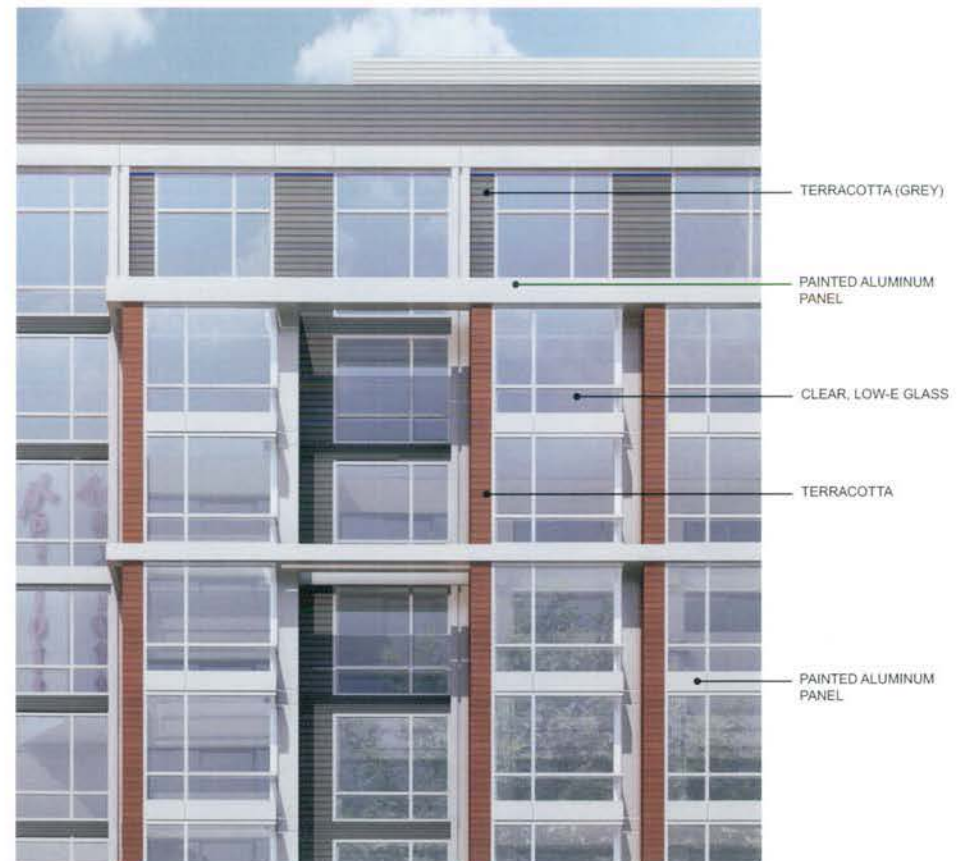
22ND STREET FACADE DETAIL
