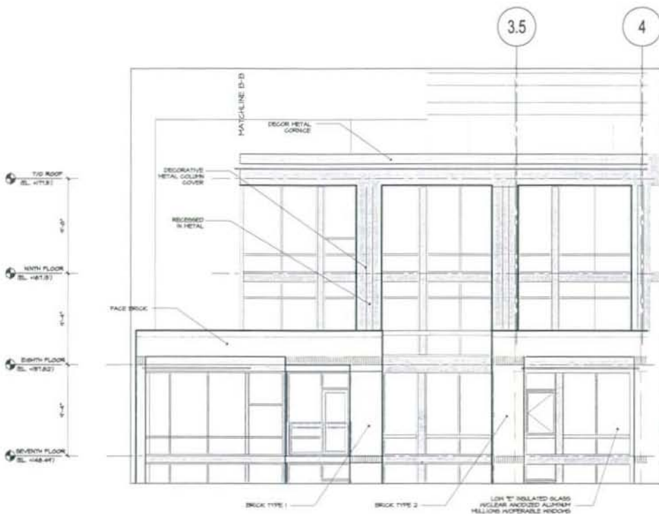
1 ENLARGED ELEVATION DETAILS SCALE: 1/4" = 1'-0"
