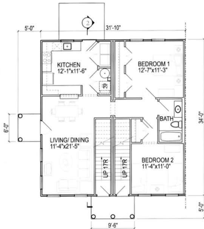
First Floor Plan First Floor Unit - 988 sf.
