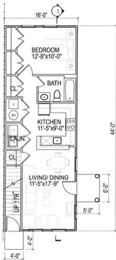
First Floor Plan First Floor Unit - 645 sf.
