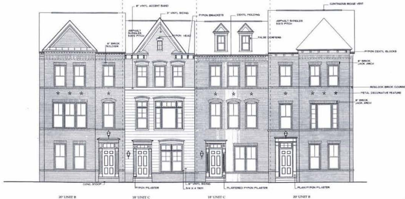
FRONT ELEVATIONS (20' ENDS, 18' INTERIORS) 1/8"=1'-0"
