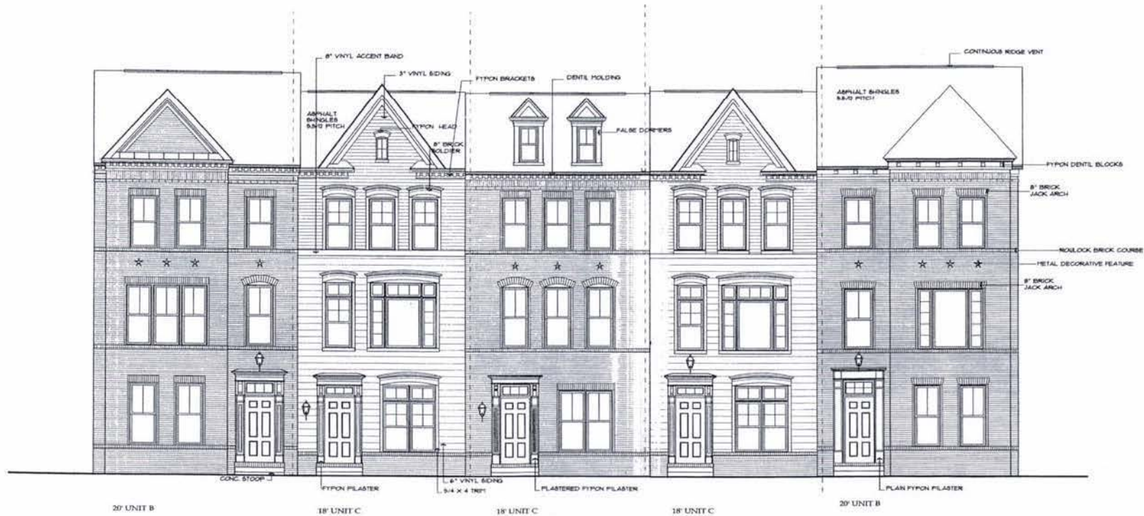
FRONT ELEVATIONS (20' ENDS, 18' INTERIORS)
