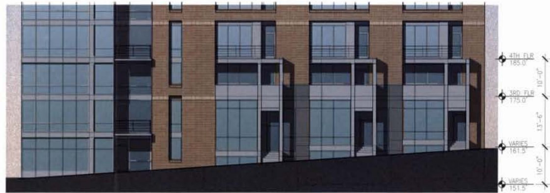
PARTIAL NORTH ELEVATION AT WALK-UP UNITS
