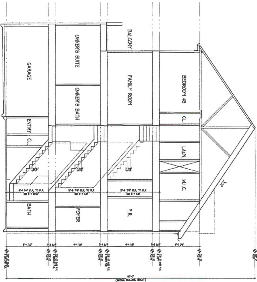
1 Building Section S-40 SCALE: 1/8" = 1'-0"
