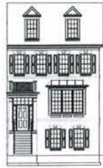
24' TOWNHOUSE UNIT B FRONT ELEVATION 4 SLAB-ON-GRADE CONDITION
