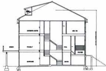
24' TOWNHOUSE UNIT B SECTION - SLAB-ON-GRADE CONDITION
