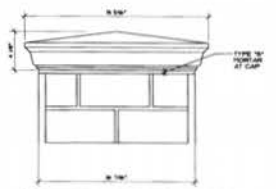
STONE PIER CAP ON 16" COLUMN SCALE: 3/4" = 1'-0"
