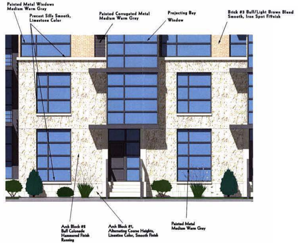
Detailed Duplex Elevation - Bldg 2
