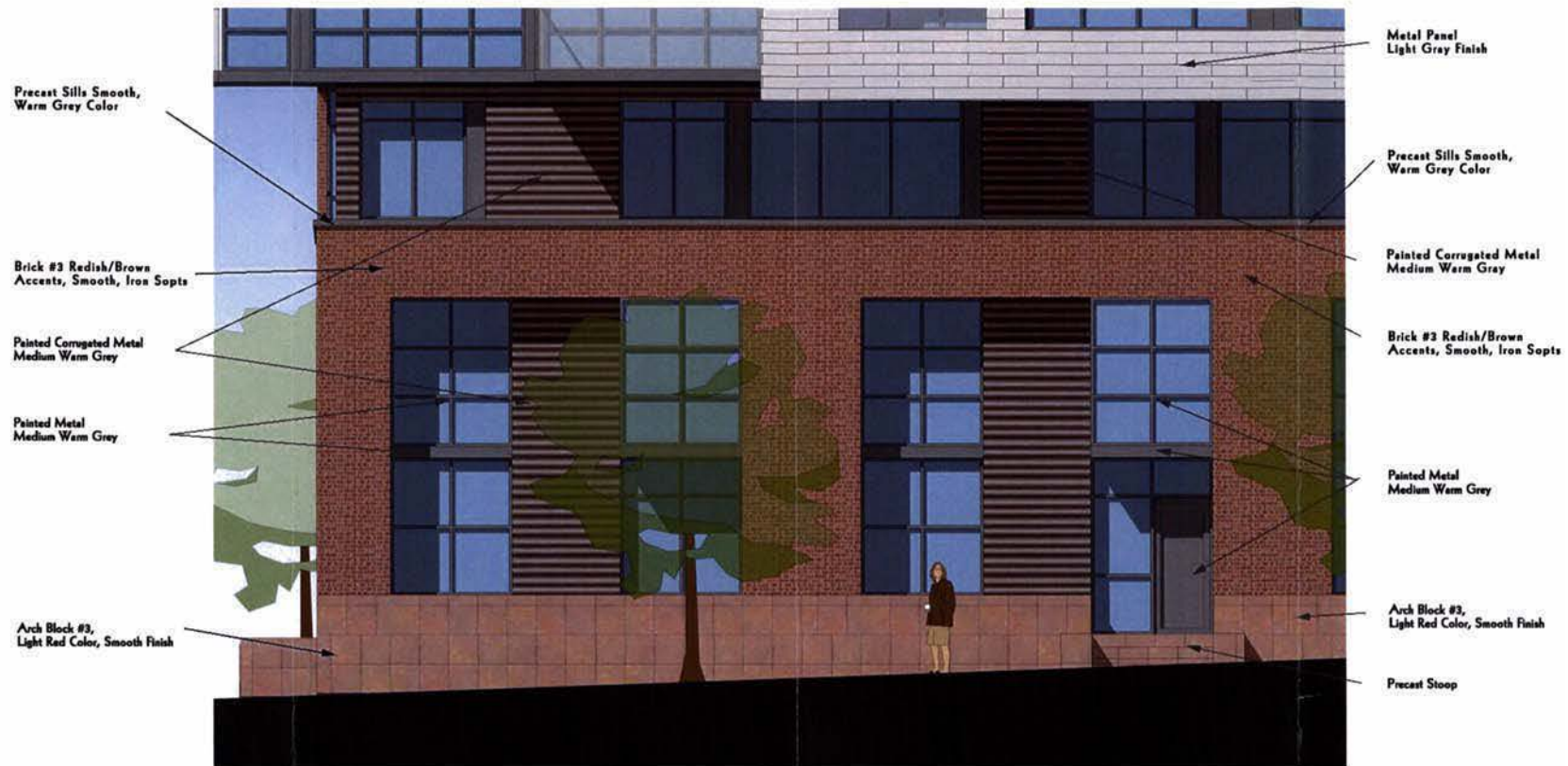
Detailed Duplex Elevation - Bldg 3
