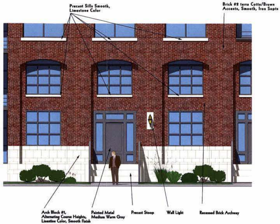
Detailed Duplex Elevation - Bldg 1
