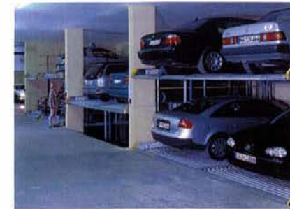
Space Saver Parking Units
