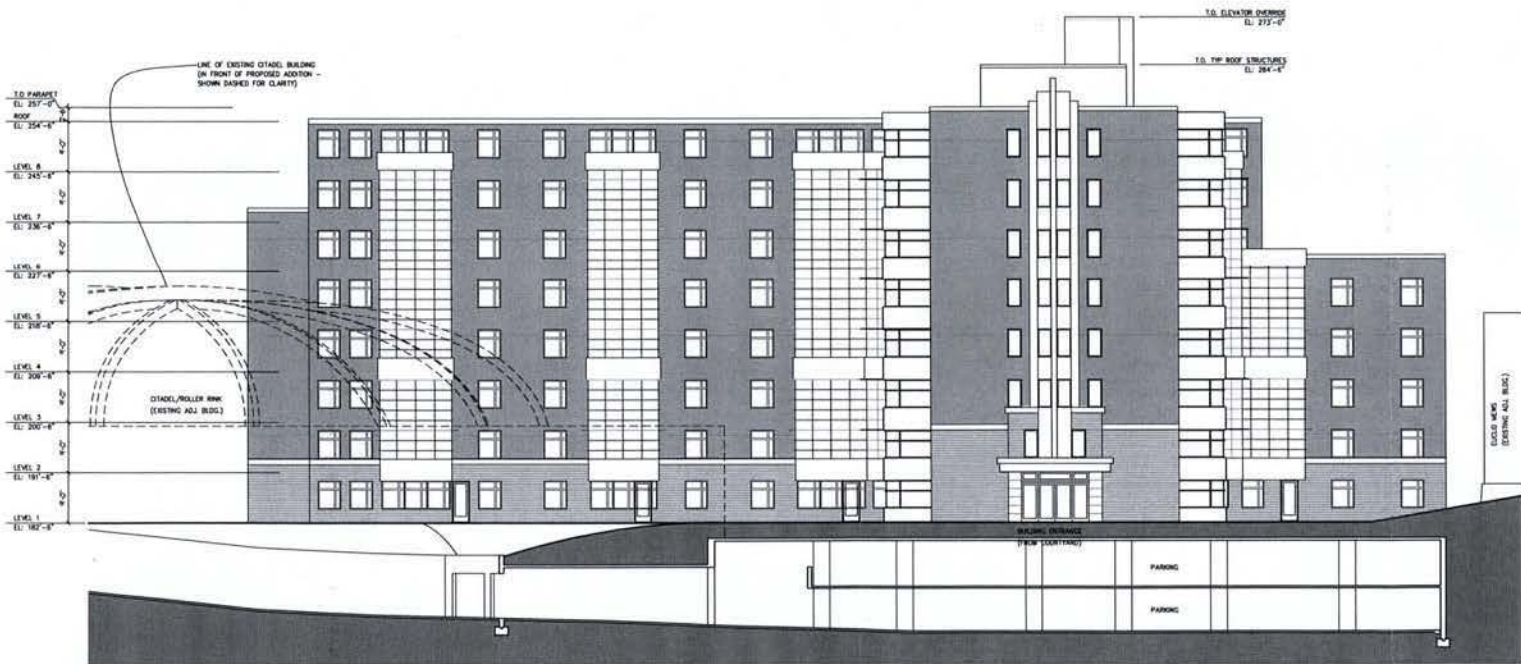
1 REAR (EAST) ELEVATION – COURTYARD ELEVATION SCALE 1/8" = 1'-0"
