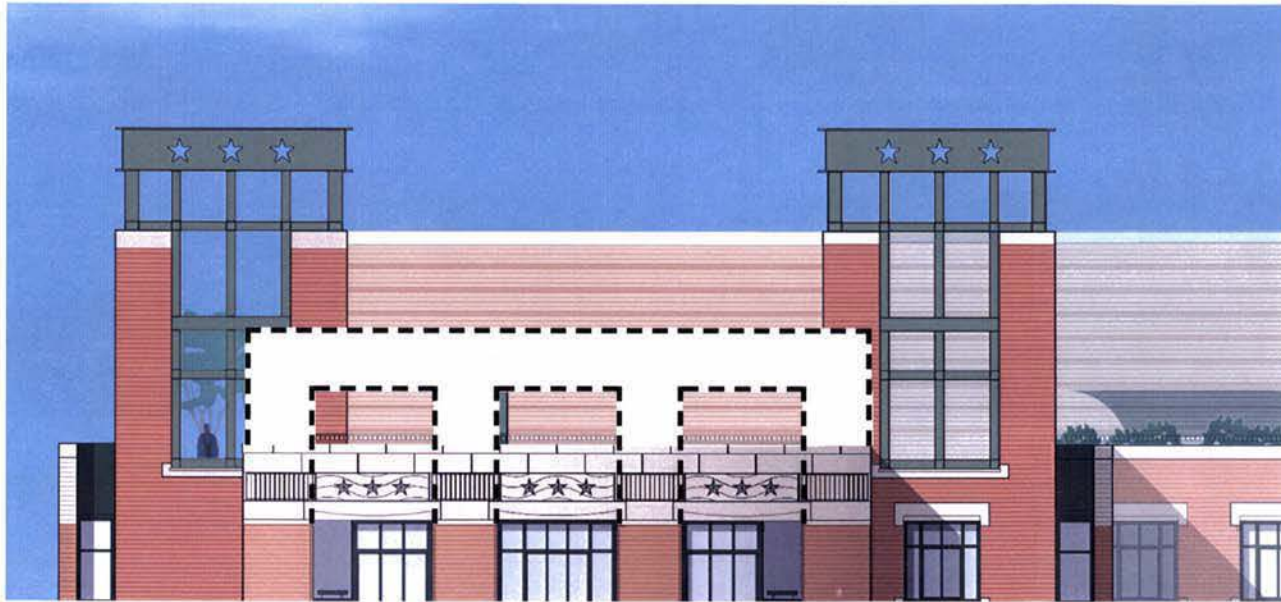
Removed screen wall tower
