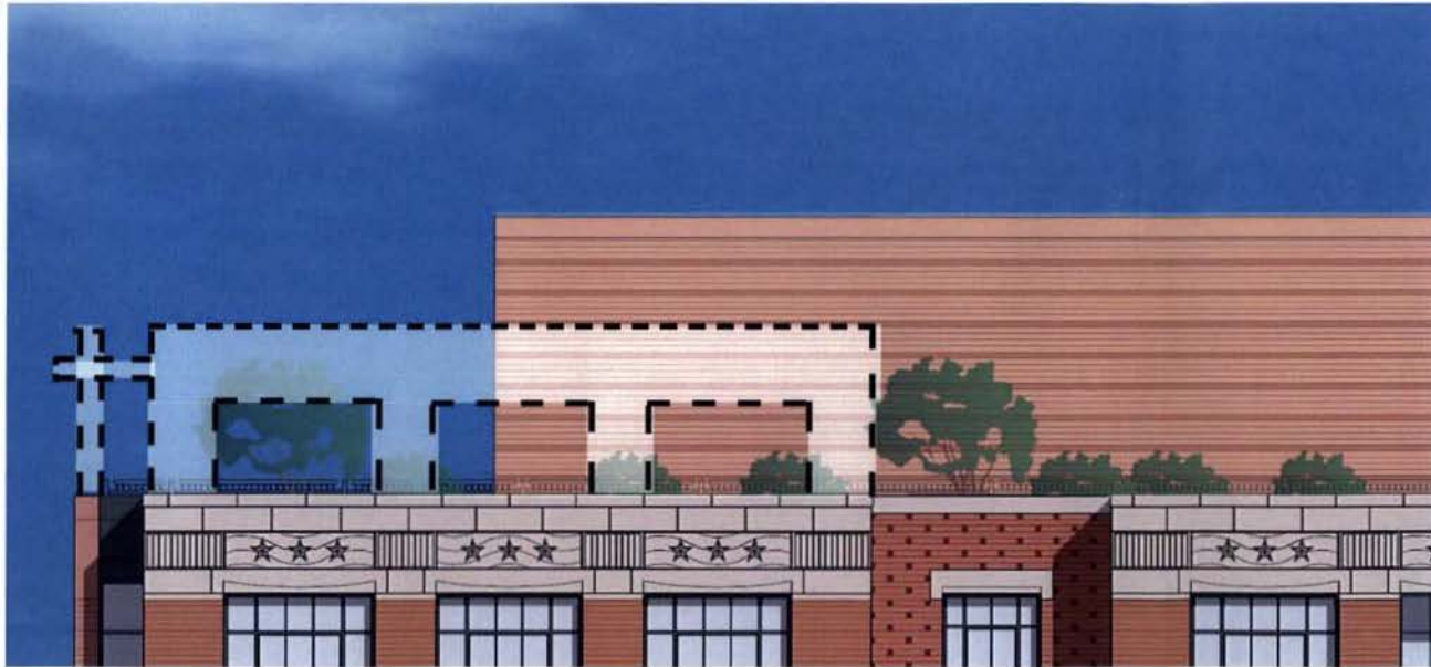
Removed three horizontal screen wall towers
