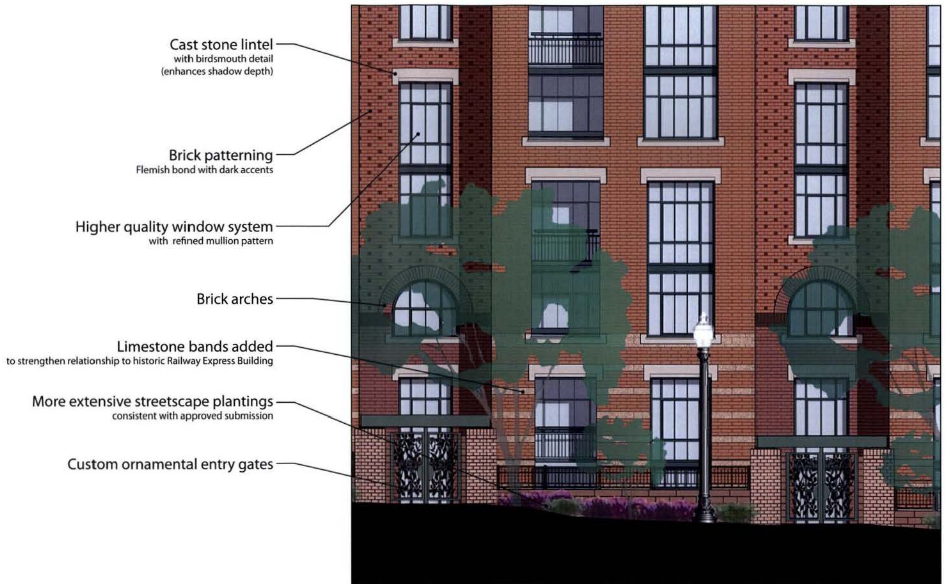
Enlarged elevation at base Second Street elevation
