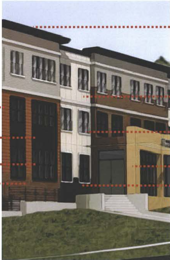
FIBER CEMENT CLADDING WITH PREFINISHED METAL TRIM
