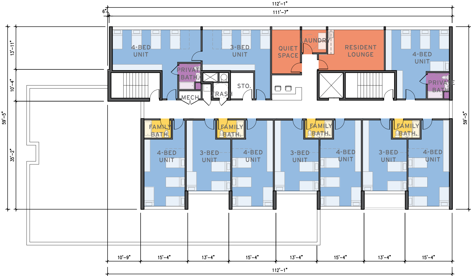
TYPICAL RESIDENTIAL FLOOR PLAN (2-4) 1/16" = 1'-0"
