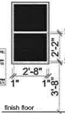
EMERGENCY ESCAPE WINDOW DETAIL SCALE: 1/4"=1'-0"
