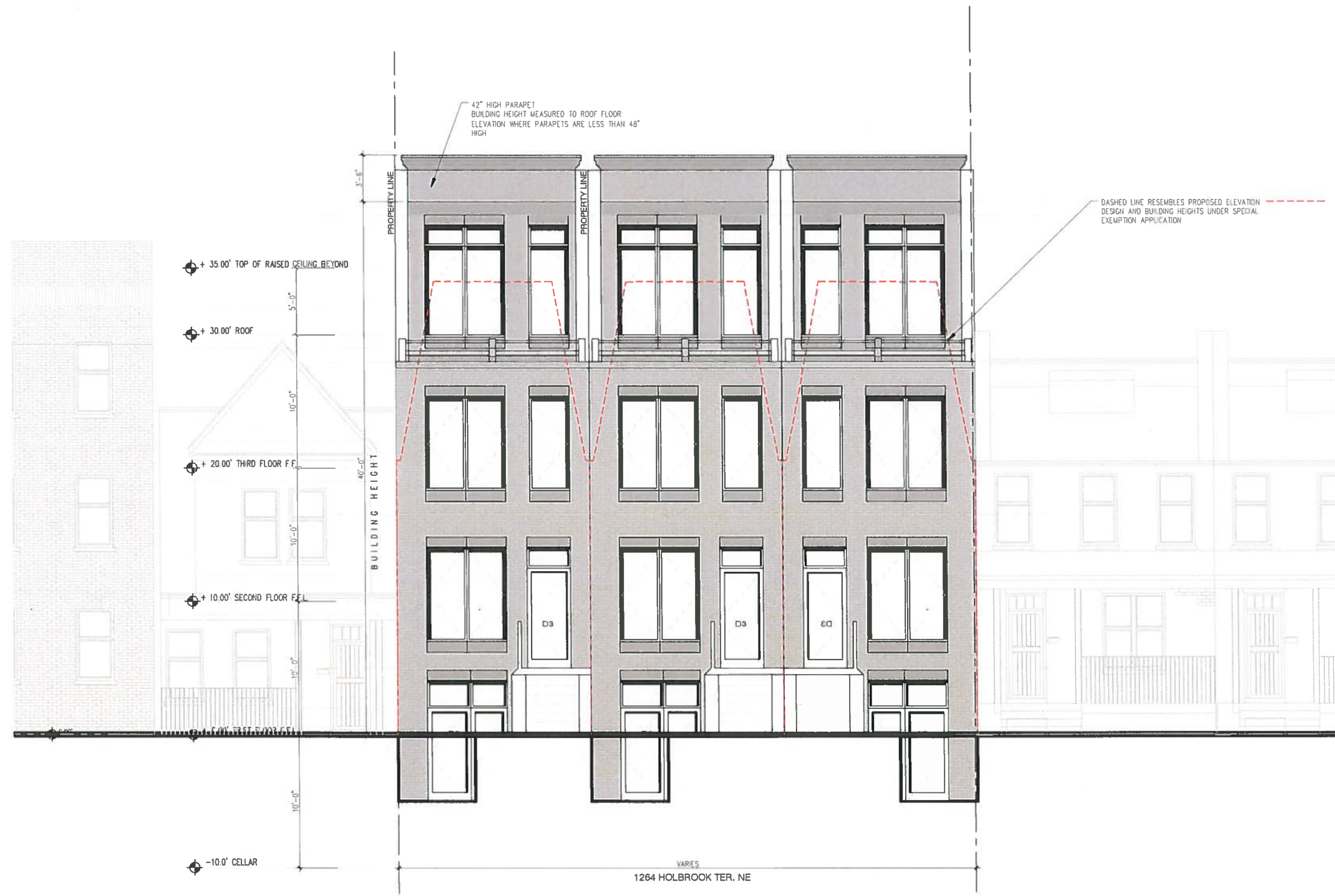
2 FRONT ELEVATION FACING HOLBROOK TER. NE SCALE: 1/4" = 1'-0"
