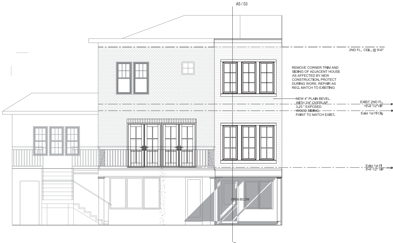
ELEVATION: REAR NEW CONSTRUCTION SCALE: 1/4" = 1'-0"
