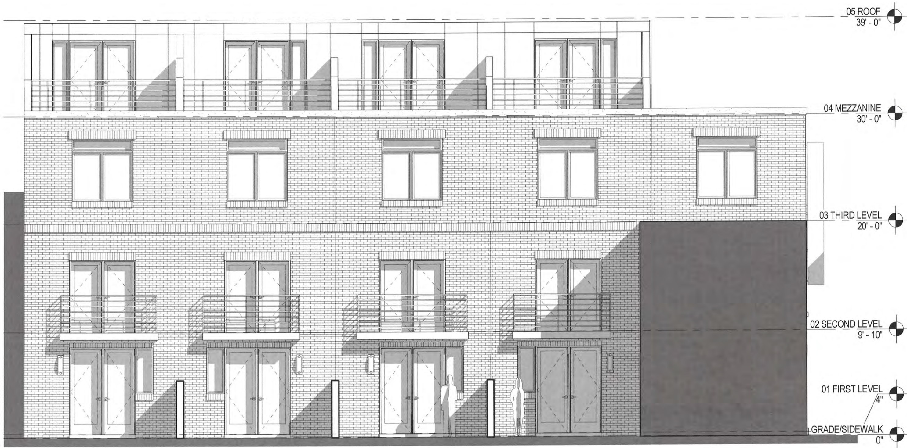
SOUTH ELEVATION - PROPOSED 3/16" = 1'-0"
