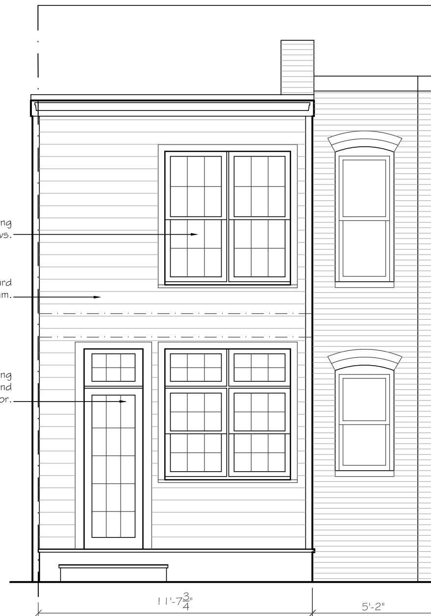
2 Proposed North Elevation A-4 1/4" = 1'-0"
