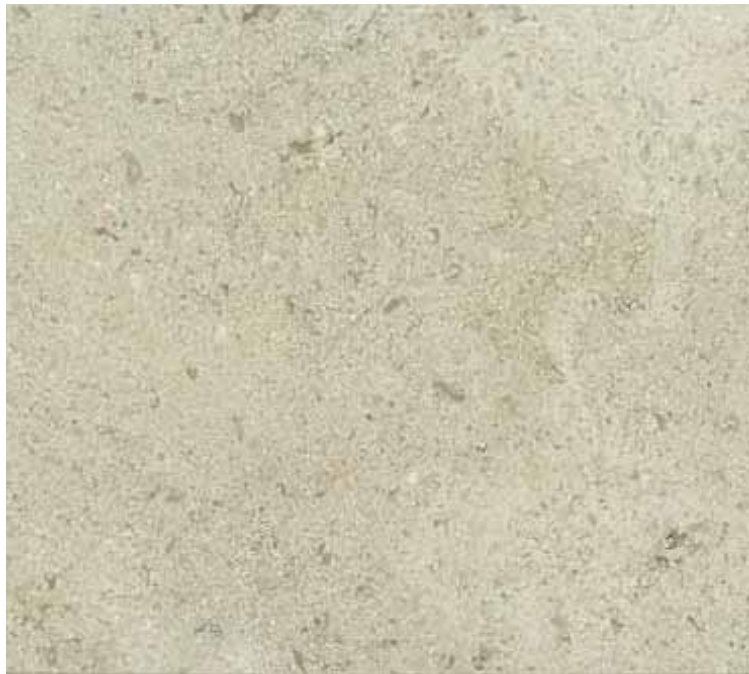
Light-colored honed limestone panels with honeycomb backing at existing precast structure (horizontal).
