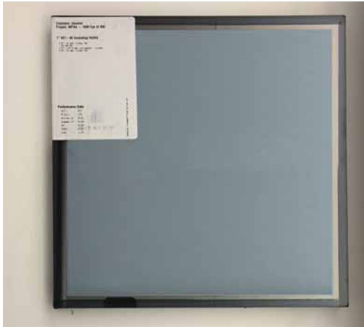
Insulated glass at typical office floors.
