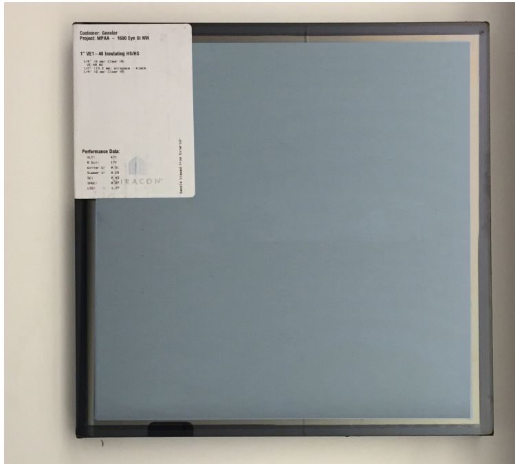
Insulated glass at typical office floors.
