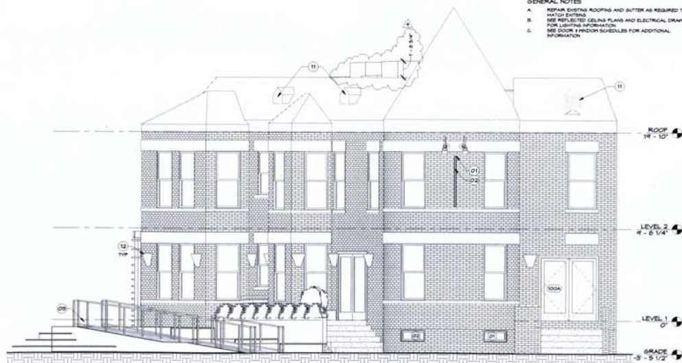
3 EXTERIOR ELEVATION - NORTH FACADE 1/4" = 1'-0"
