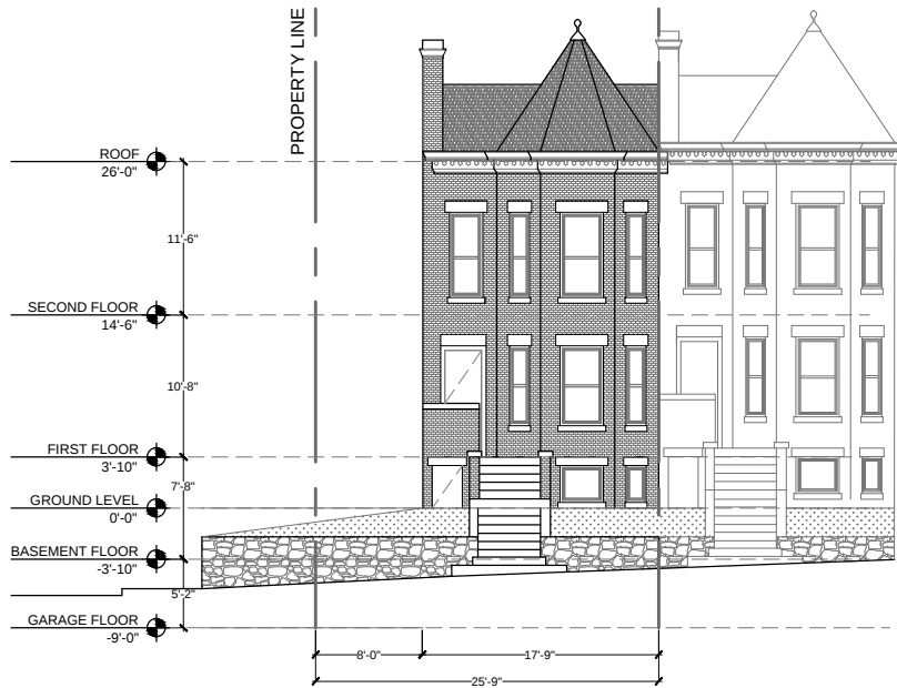
2 A0.2 EXISTING BACK ELEVATION 1/16"=1'0"
