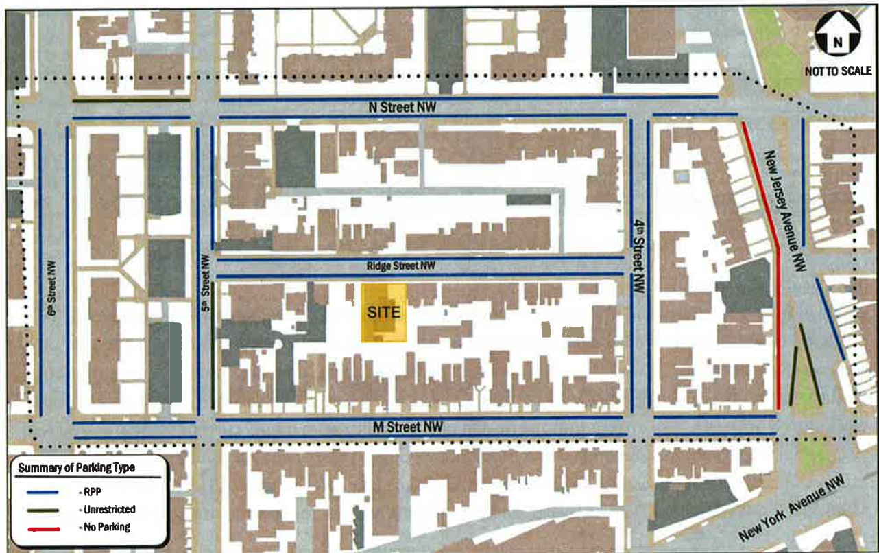
Figure 2 Parking Restrictions (Source: Grove/Slade)
