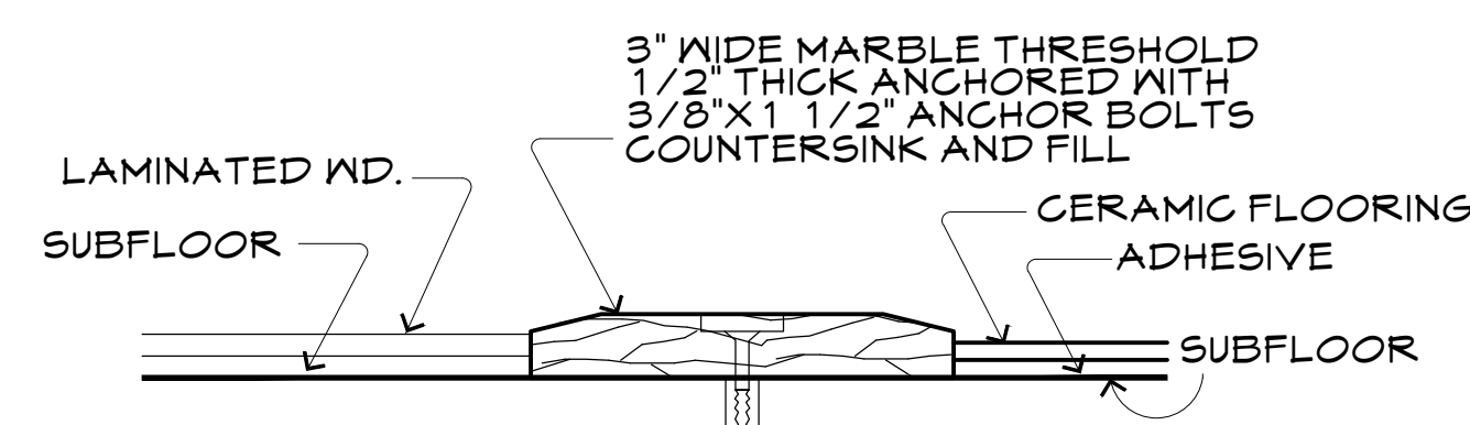
BATHROOM DOOR SILL (TYPICAL) NOT TO SCALE
