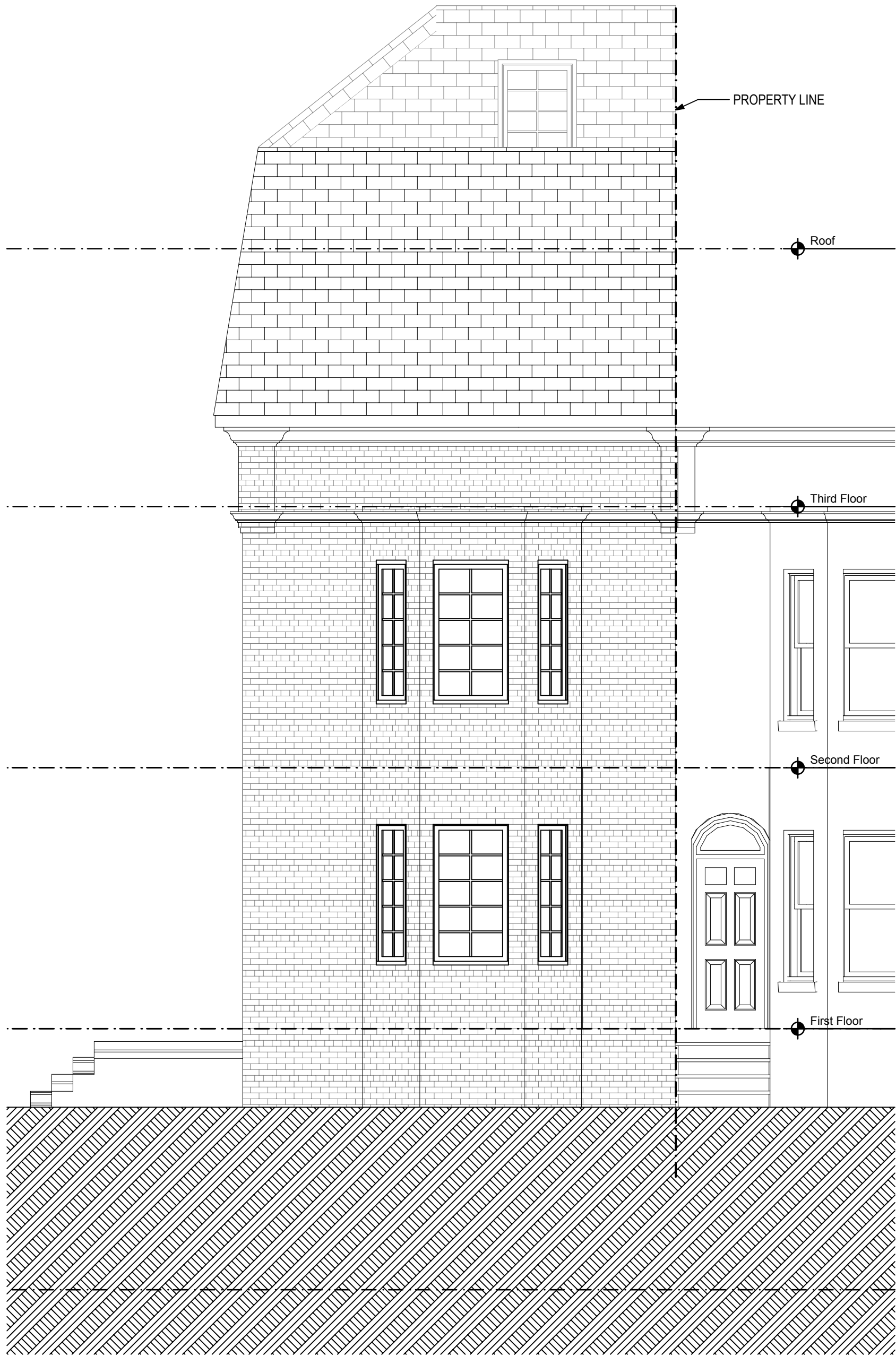
1 Front Elevation SCALE: 1/4" = 1'-0"
