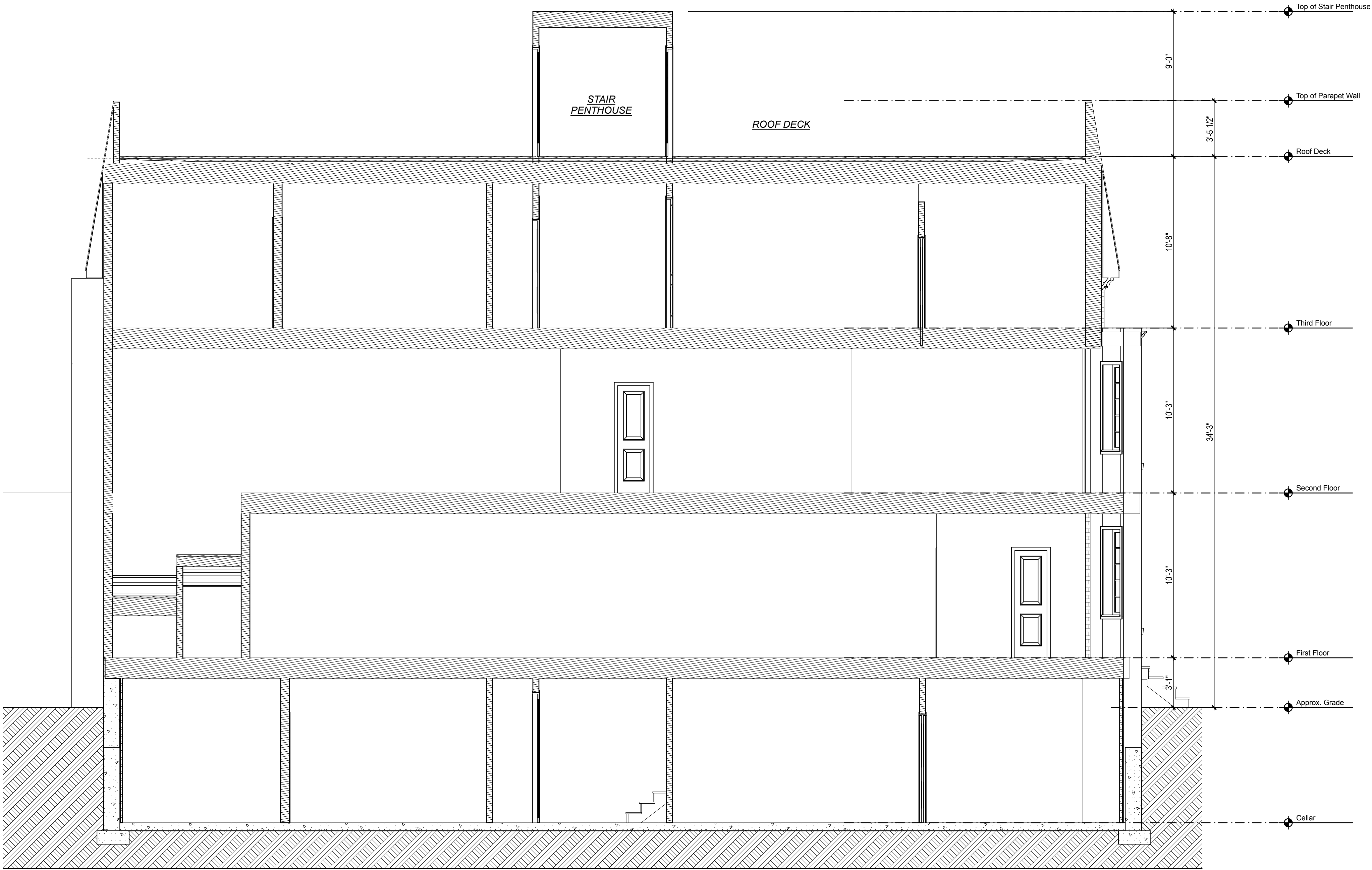
1 Building Section 2 SCALE: 1/4" = 1'-0"
