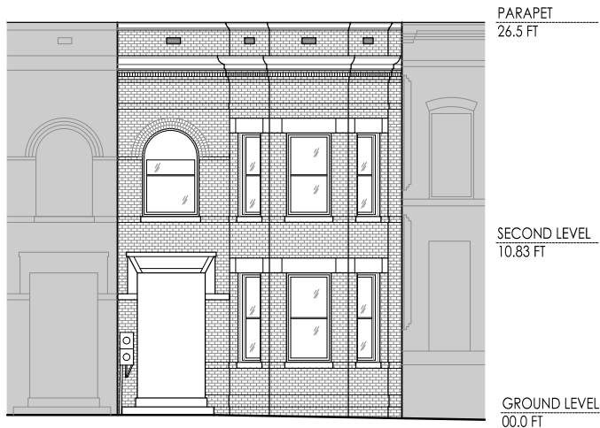
1 EXISTING EAST ELEVATION (FRONT) 1/4" = 1'-0"
