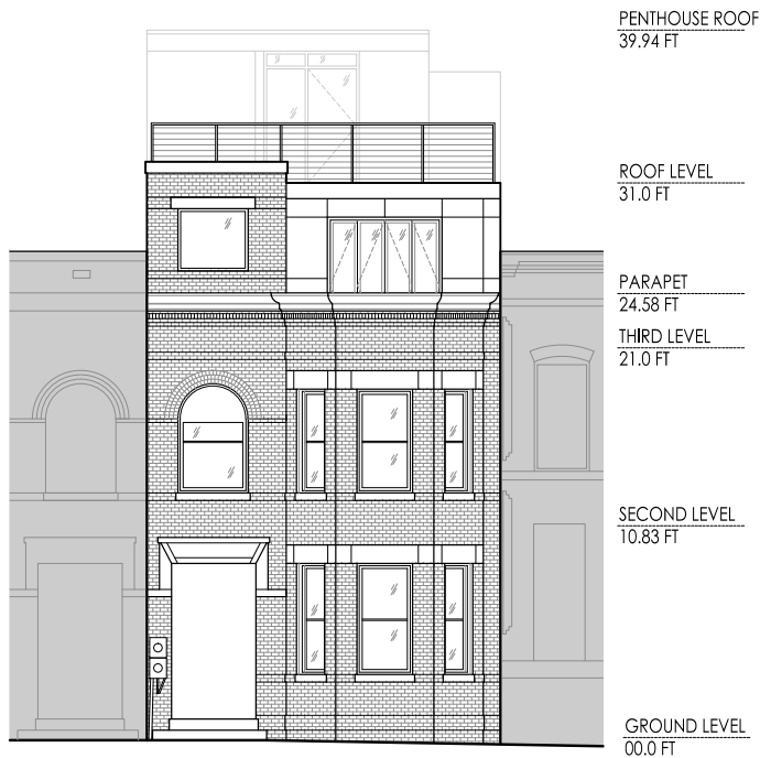
2 EAST ELEVATION (FRONT) 1/8" = 1'-0"
