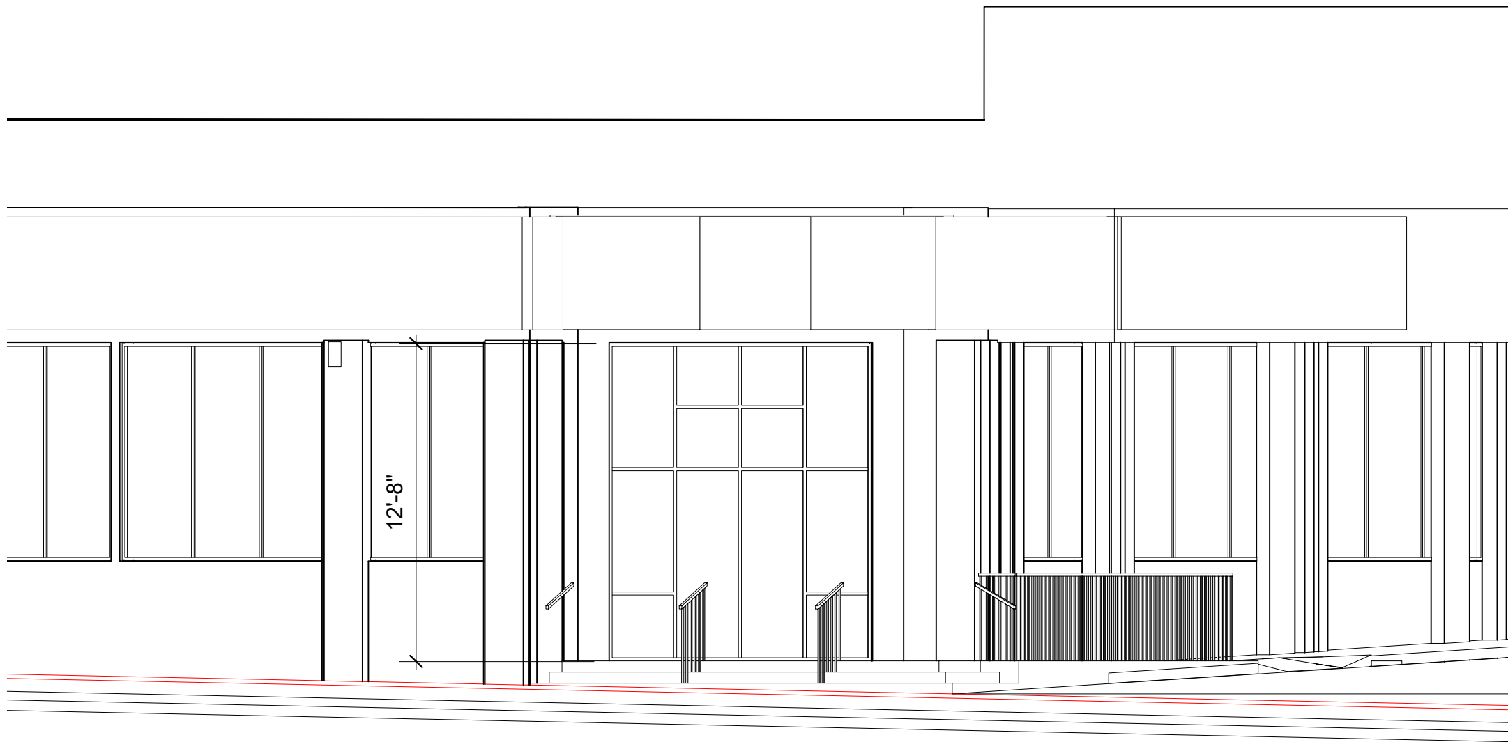
NORTHWEST: Kawneer 451T Bronze Aluminum Storefront Sytem with 1" insulated clear glass
