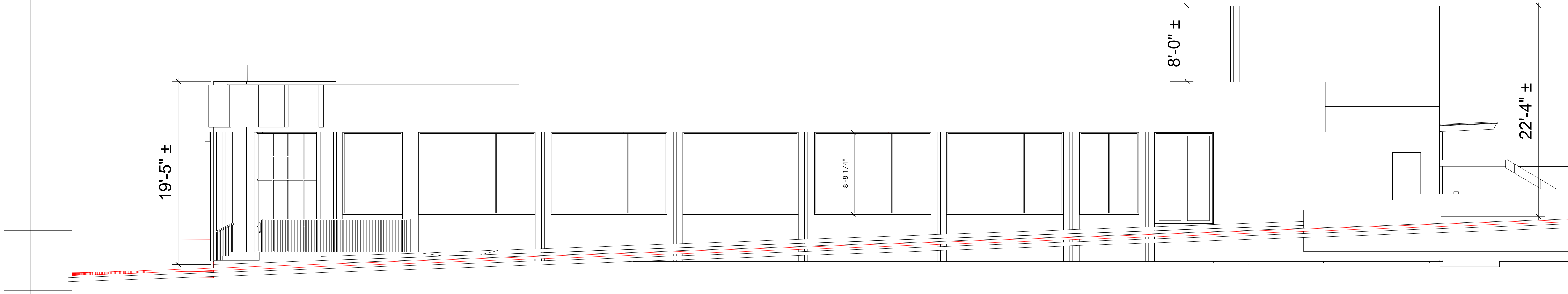
WEST: Kawneer 451T Bronze Aluminum Storefront Sytem with 1" insulated clear glass
