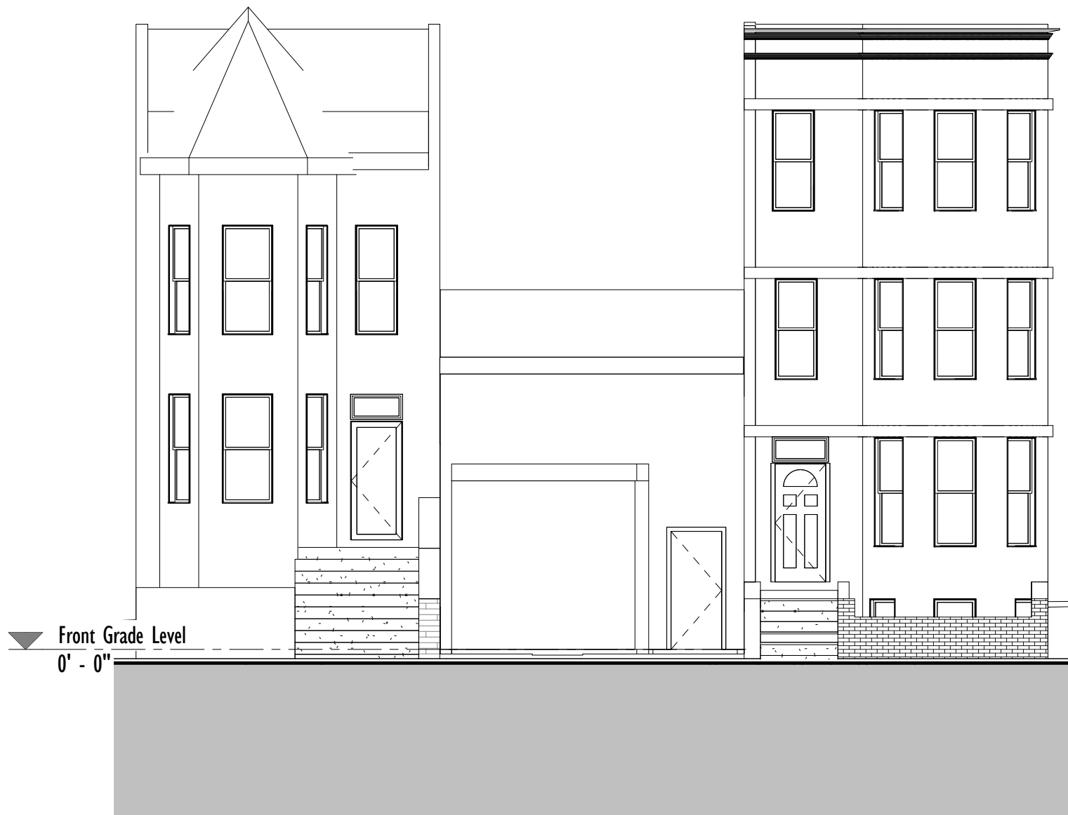
② Existing Front Elevation 1/8" = 1'-0"
