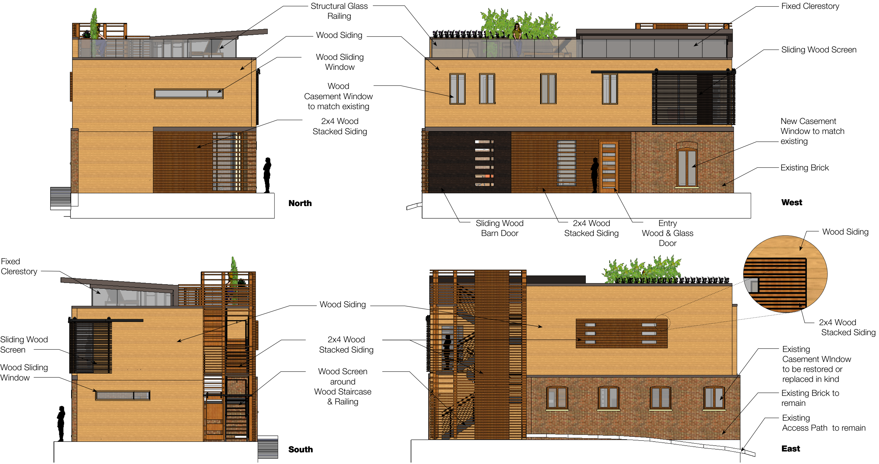
Exterior Elevations - Closed - 1/8" = 1'-0"
