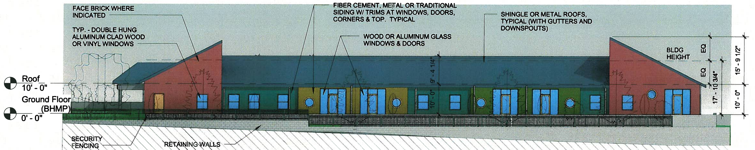
2 WEST (4TH STREET) ELEVATION A-201 SCALE 1/16" = 1'-0"
