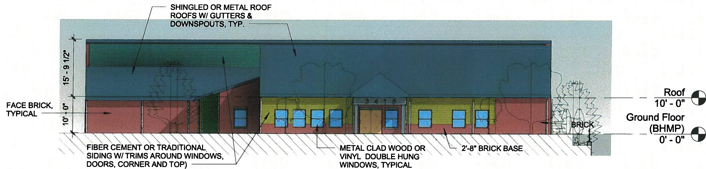
1 NORTH (FRONT) ELEVATION A-201 SCALE 1/16" = 1'-0"
