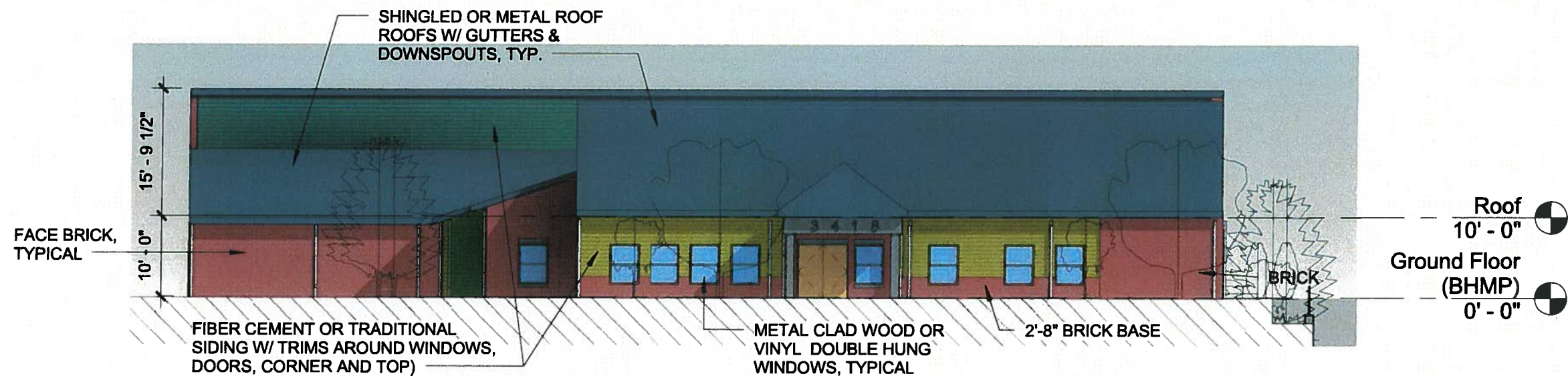
1 NORTH (FRONT) ELEVATION A-201 SCALE 1/16" = 1'-0"
