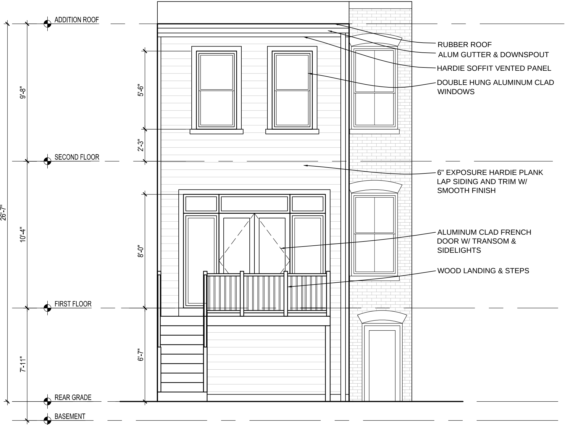
1 A-4 PROPOED REAR ELEVATION SCALE:1/4"=1'-0"
