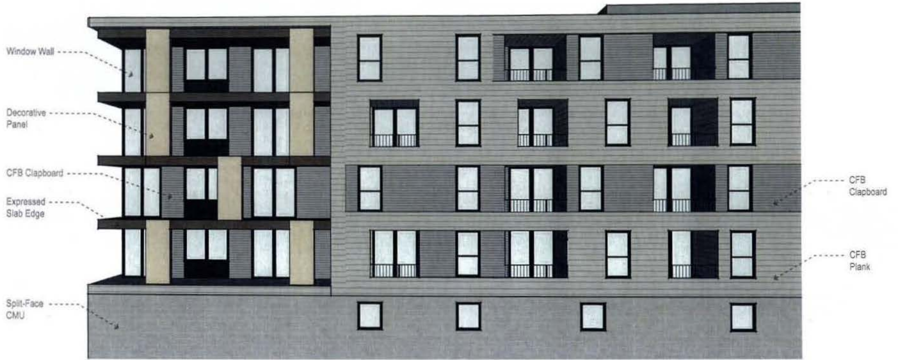
A: BUILDING ELEVATION
