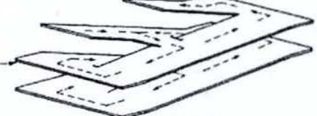
SLOPING FLOORS-CROSS CONNECTION ONE-WAY CIRCULATION
