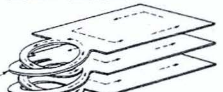
CONCENTRIC OPPOSED PLANE HELICAL RAMP
