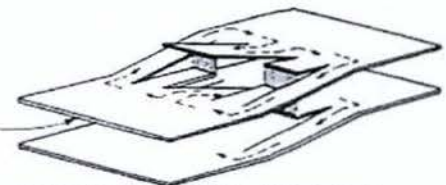
STAGGERED FLOORS-TWO-WAY CENTER RAMP
