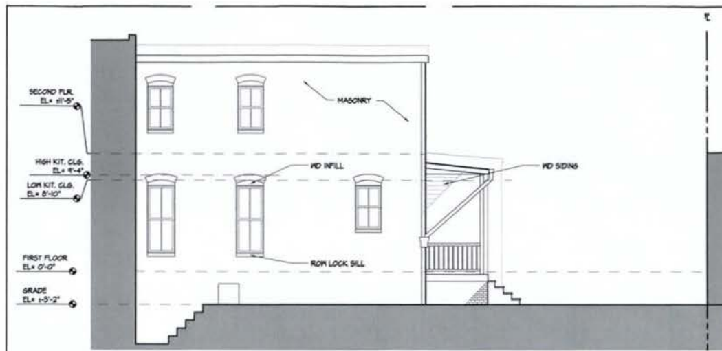
1 EXISTING SIDE ELEVATION 1/4" = 1'-0"
