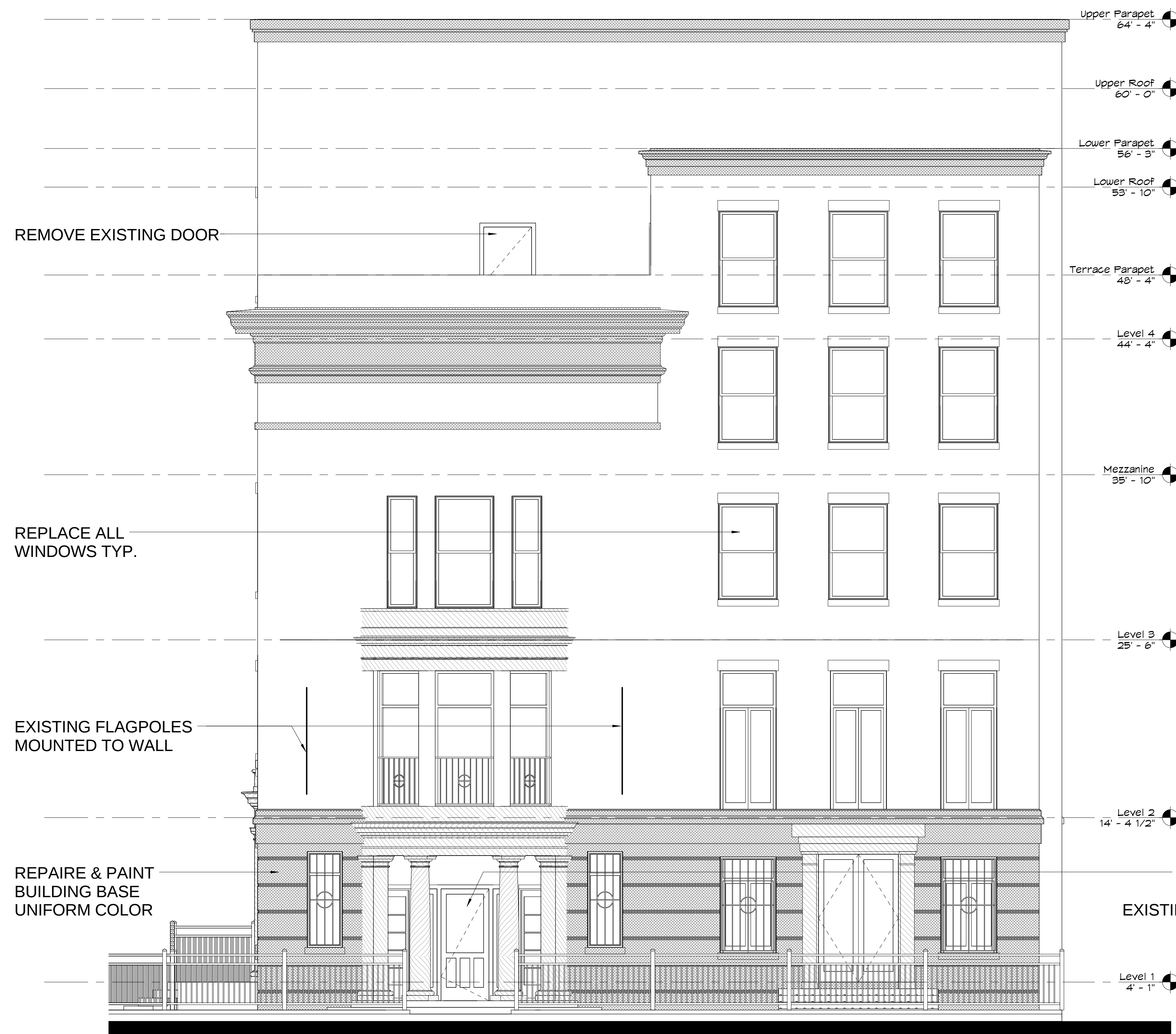
① EAST ELEVATION - EXISTING 1/4" = 1'-0"
