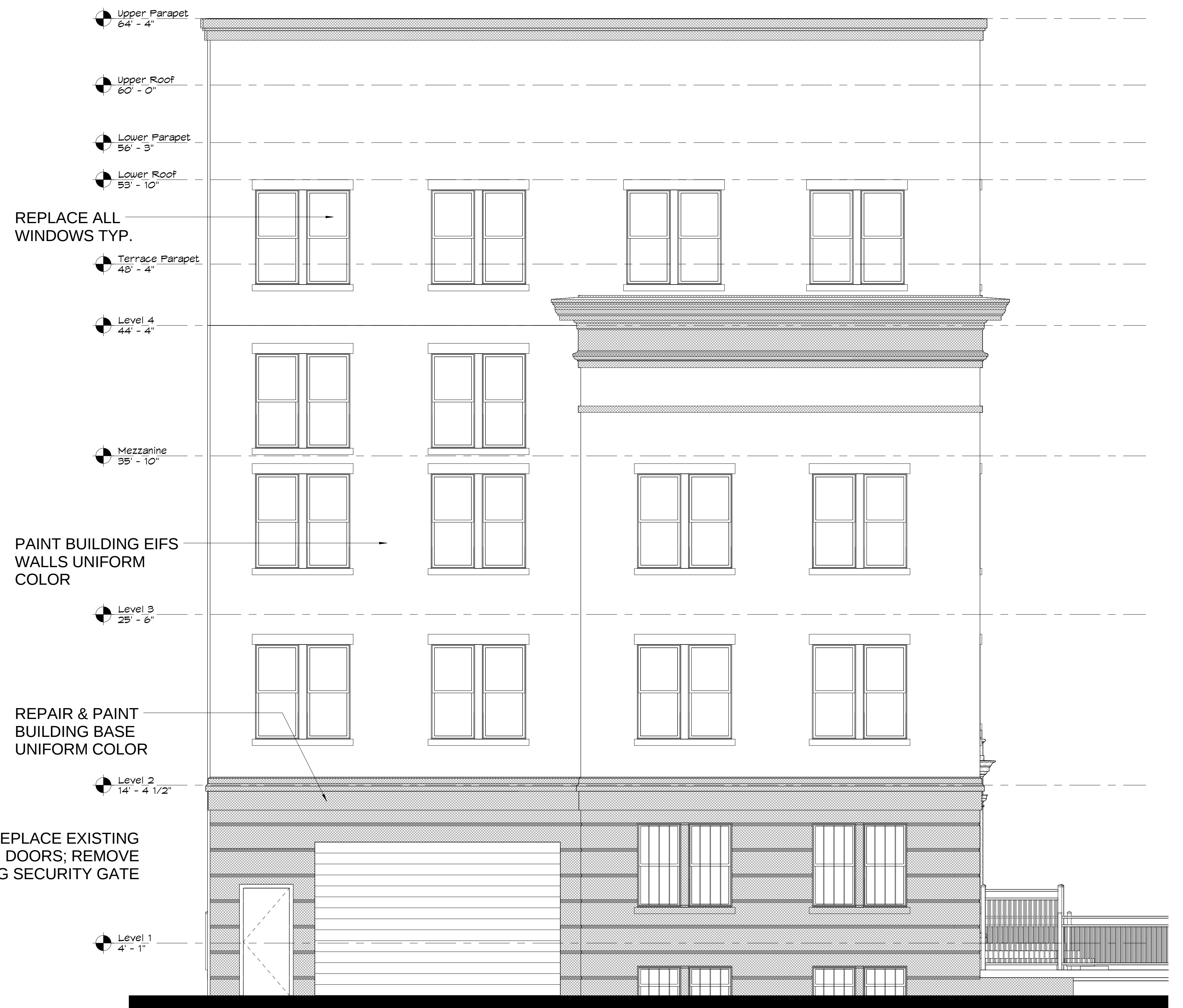
② WEST ELEVATION - EXISTING 1/4" = 1'-0"
