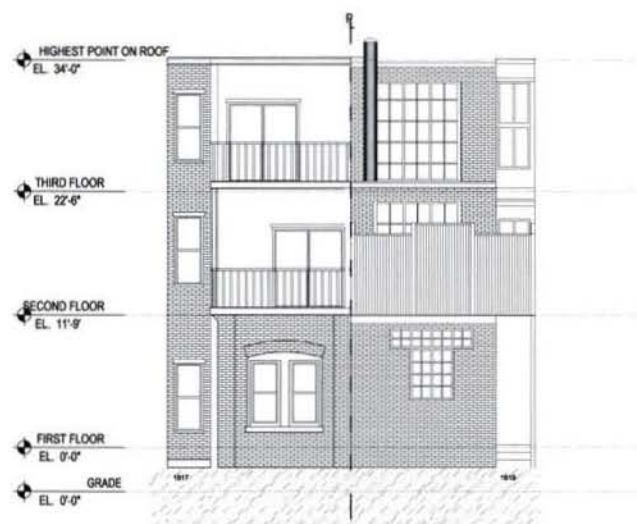
2 EXISTING REAR ELEVATIONS SCALE: 5/32"=1'-0"
