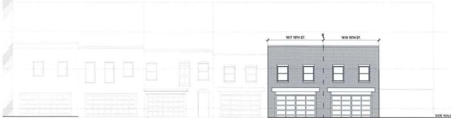
3 PROPOSED ELEV. W/ADJ. BLDGS. SCALE: 3/32"=1'-0"
