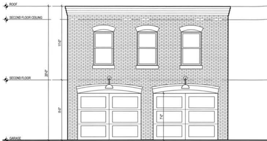
2 WEST ELEVATION GARAGE ADDITION A-9 SCALE: 3/16"=1'-0"
