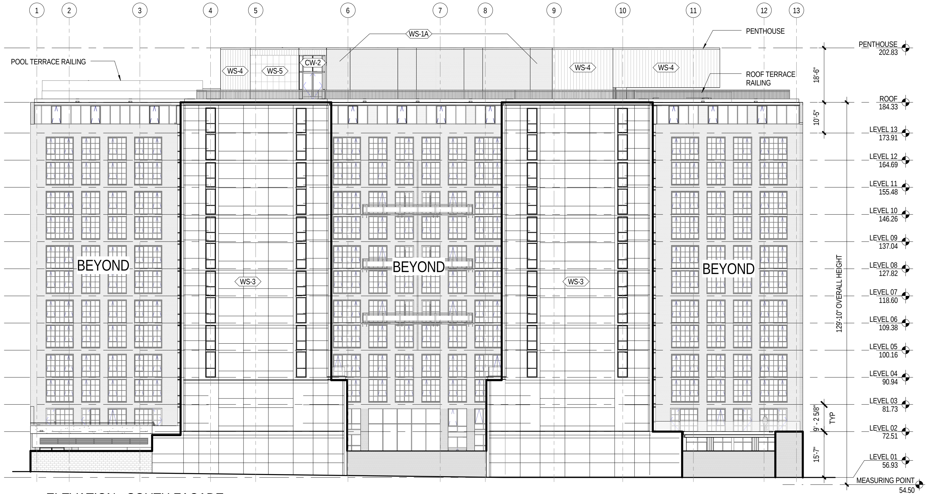
1 ELEVATION - SOUTH FACADE
