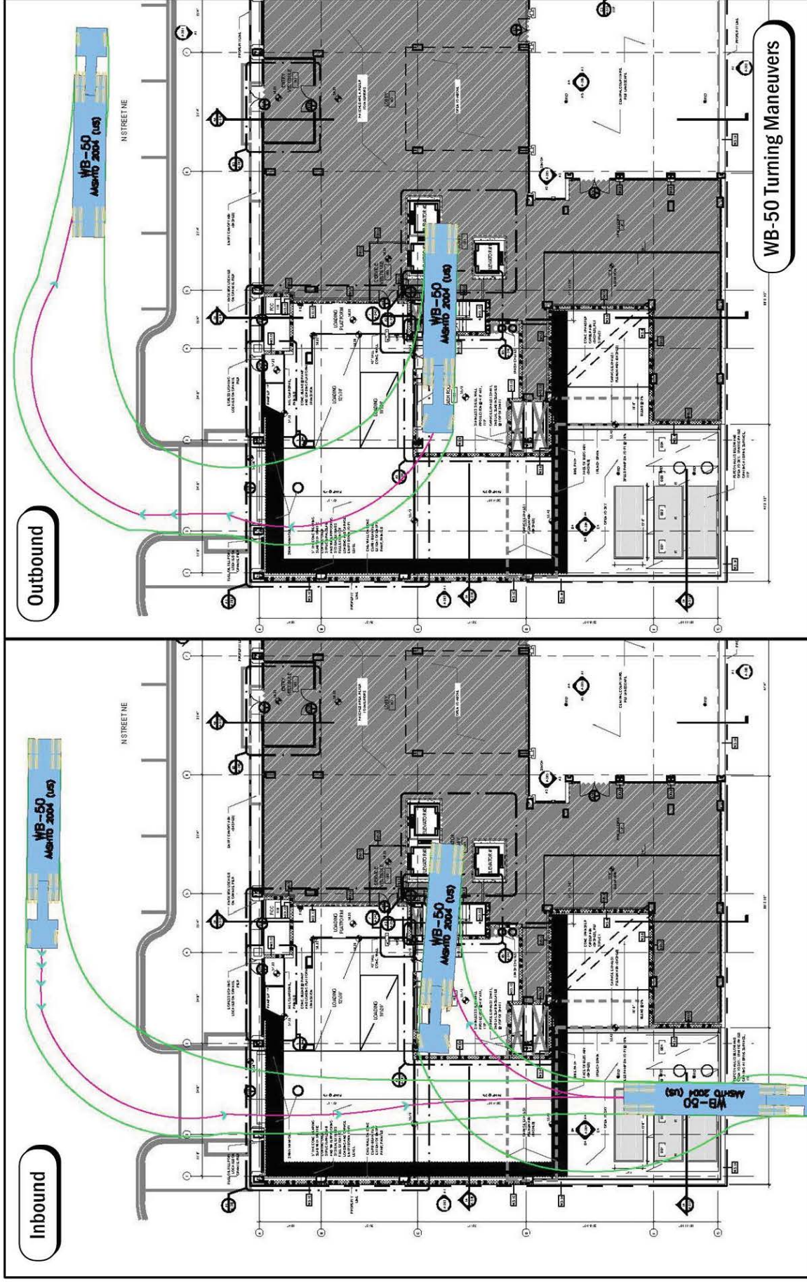
Figure 4: 55 Foot Truck Turning Maneuvers
